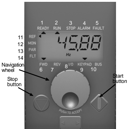
Figure 7.11: Vacon 10 Control panel
